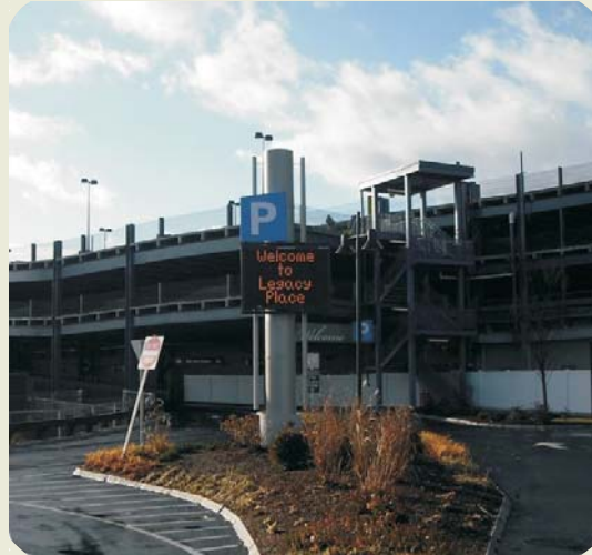
Large variable message sign used for marketing or parking information.
