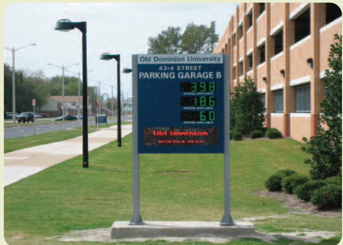
Dynamic signs at key decision making points help parkers locate the nearest available space.
